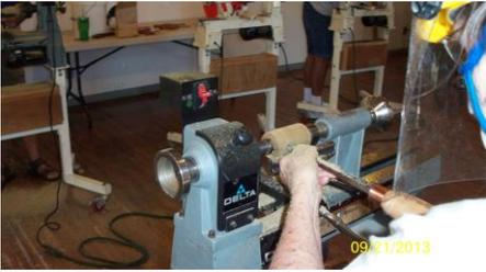
Spindle turning with Easy Wood Tool
