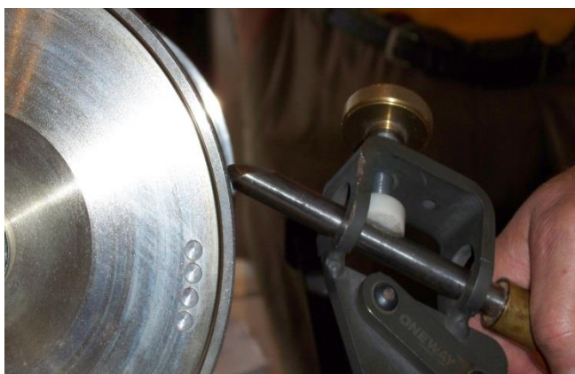
Raptor Set Up Tool – Used to determine correct angle for sharpening various tools, as shown in picture at right. 5 piece set has angles of 35, 40, 45, 50 & 60 degrees. (60 degree angle shown)
