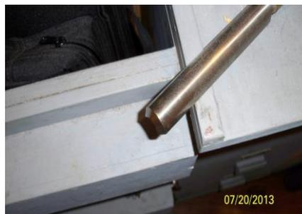
Correctly sharpened – back view
