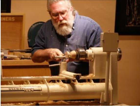
Using a three-axis jamb chuck
